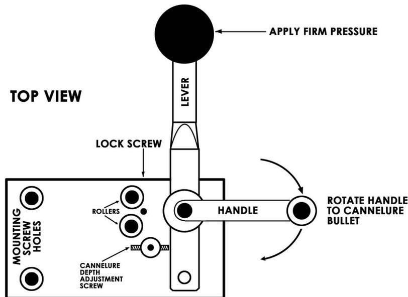
1. Base must be held firmly by attaching to bench or clamping in a vice.
